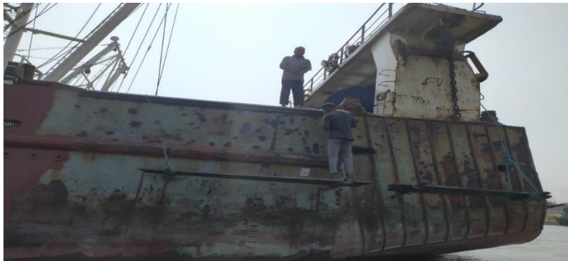
Figure 1 : Removing paint from ship ( picture captured by researcher )
