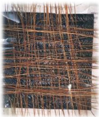
(a) Collected Areca Nut Leaf Sheath Fiber (10% Alkali treated)
