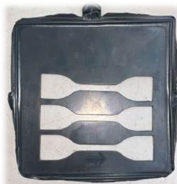
(b) Sample cut from galvanized matt manual cutting machine
