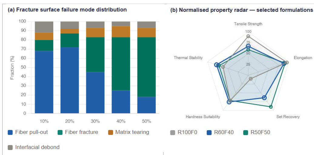
Fig. 3. (a) Fracture surface failure mode distribution from SEM fractography across five fiber-containing formulations. The transition from pull-out-dominated (68% at 10 wt%) to fracture-dominated (58% at 40 wt%) failure is consistent with the onset of mechanical strength recovery above 30 wt%. (b) Radar chart of normalised mechanical properties (tensile strength, elongation, permanent set recovery, hardness suitability, thermal stability) for three representative formulations. R60F40 presents the most evenly distributed profile across all five performance axes.
